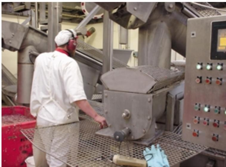
*Employee at the screw conveyors, which are covered by mesh to prevent accidents.
