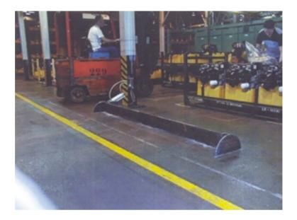
entering the work area until the operators have moved to the next bay. The last operator in the area lowers the barrier and sets off audio and visual alarms to ensure that no operator enters the area. Lights are used to indicate to the driver that the bay has been evacuated and they can enter to remove racks of completed engines and replace the empty racks. The prevention process involved:
