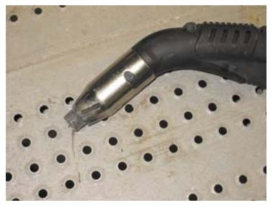
Integrated extractor fitted to MIG welding gun
