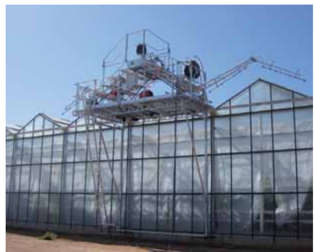
The Repair Shuttle enables repairs to be made to glasshouses safely and quickly
