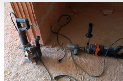
Good practice: Extracted hand machines: The illustration shows 2 extracted hand machines used for cutting and drilling work.
