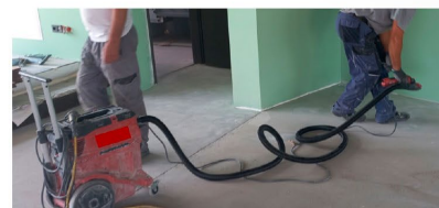
Good practice: Extracted hand machines: The illustration shows 2 extracted hand machines used for cutting and drilling work.
