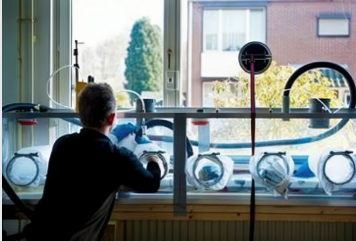
Figure 8-3: Examples of glove boxes
