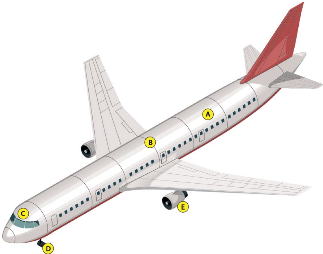
Figure 14-5: Aircraft – where asbestos might be found (non-exhaustive)
